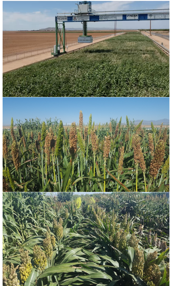
Figure 1: The TERRA-REF Field and Gantry-based Field Scanner in Maricopa, Arizona (top), with sorghum being grown in the field. Sorghum is a hugely important cereal crop, widely used as a source of grain, agricultural feed, and even bio-fuel. Over several seasons, hundreds of varieties of both bio-energy and grain sorghum were grown in the TERRA-REF field (middle and bottom), and were imaged daily for the purpose of high throughput phenotyping.
